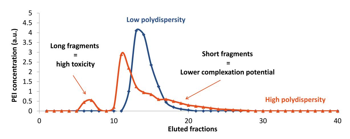
Optimization process of PEI polymer chemistry. Whereas long polymer fragments lead to cell toxicity and short fragments lead to lower complexation potential (in red), optimized PEI size with a low polydispersity index decreases toxicity, while increasing complexation potential (in blue) and reproducibility in transfection.
