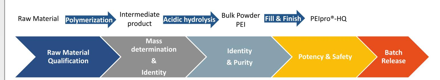
Manufacturing process of PEIpro® and PEIpro®-HQ reagents. The linear structure of PEIpro® and the manufacturing process developed by Polyplus-transfection® ensure a high, stable and reproducible amount of protonable amines available for transfection while providing a fully deacylated molecule and an extremely low polymer chain length variation.
