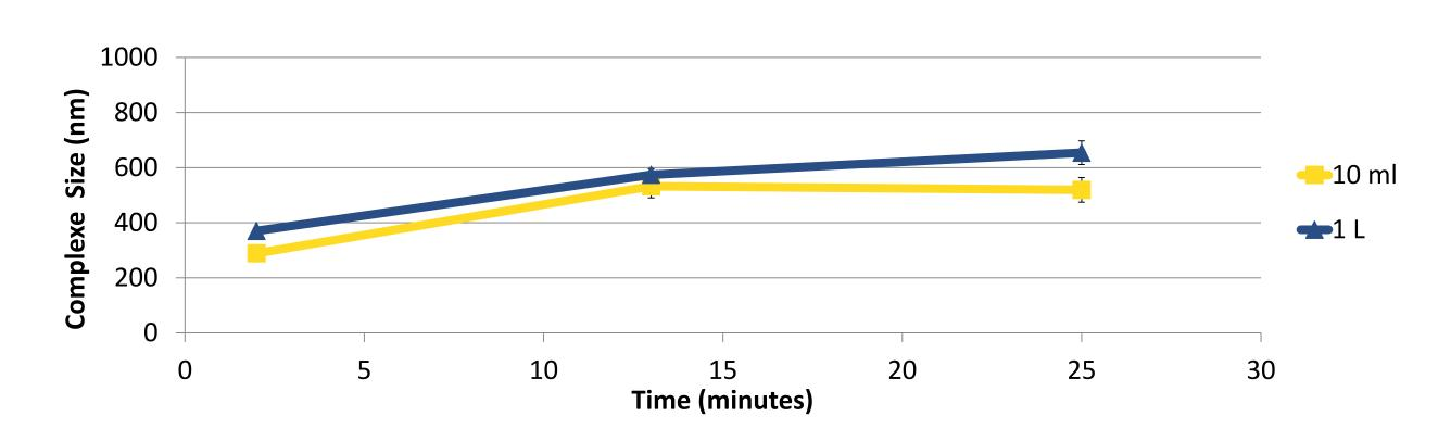
DNA-PEIpro® complex size is identical, independently from the volume of transfection mix preparation. Complexes were prepared with a DNA concentration of 0.01 mg per mL of complex volume at a DNA:Reagent ratio of 1:4, either in 10 mL or 1 L. The size of the complexes was then measured every ten minutes using the Zetasizer Nanometer ZS (Malvern Instrument, Malvern, UK).
